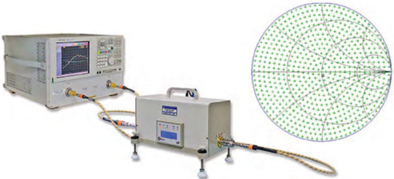
Figure 3. An automated slide-screw impedance tuner setup with a calibrated VNA and automated software.
